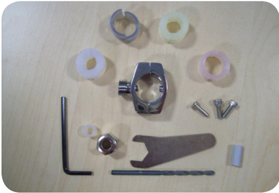
Metal saddle kit R0640004 For pipe work with a diameter ranging from 10 to 16mm 3mm drill bit needed for installation. Included in with kit
